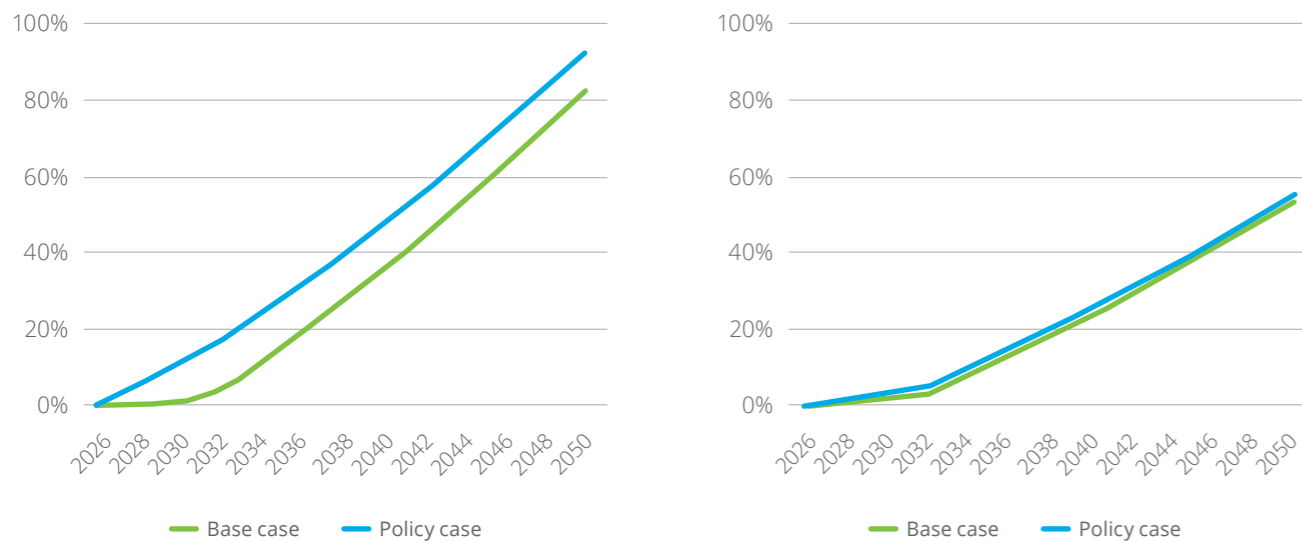
Chart 3.3: Electric share of rigid truck fleet (left) and articulated truck fleet (right)
